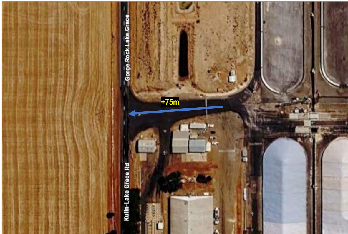
Figure 20: Approach Sight Distance Measurement – CBH Site Exit to Kulin-Lake Grace Road
