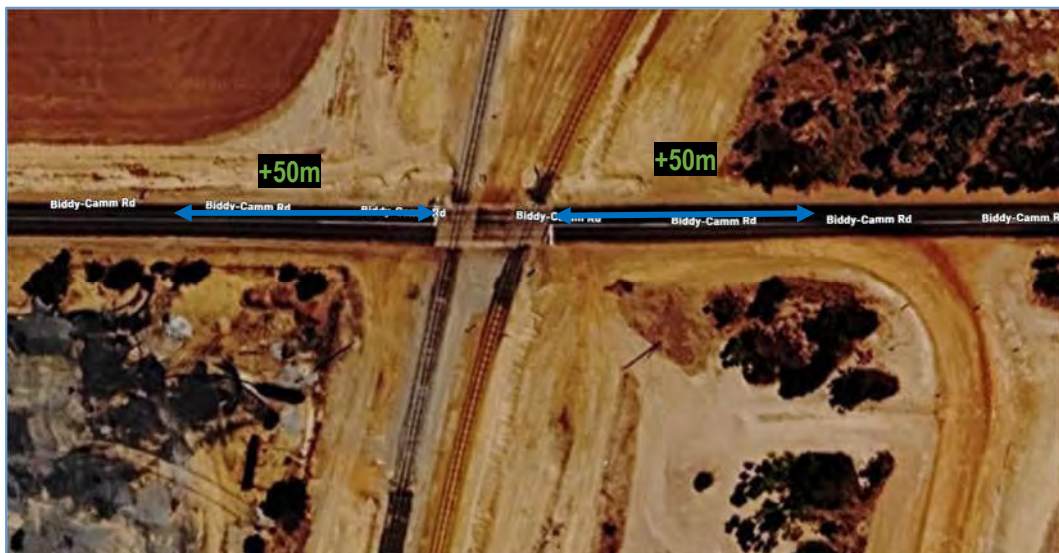
Figure 39: Stacking Distance – Biddy-Camm Road Level Crossing
