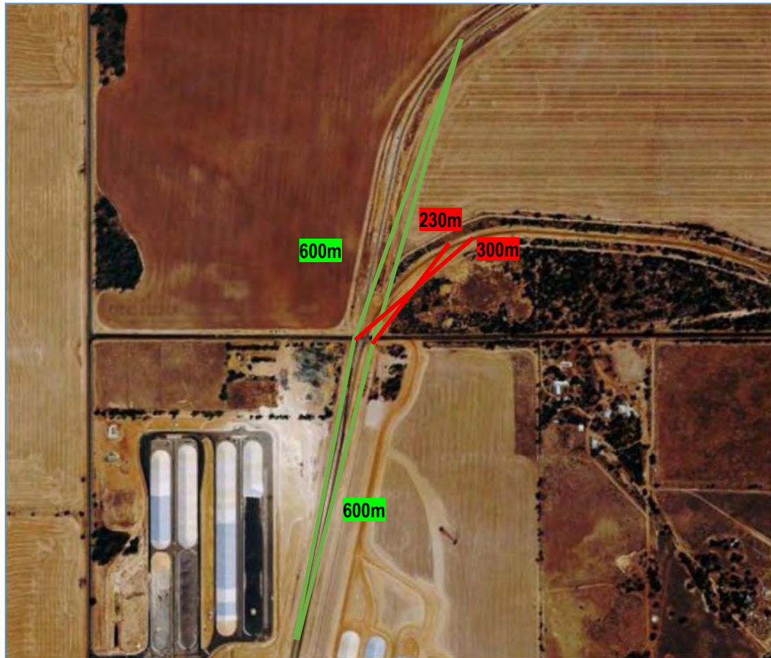
Figure 45: Available Sight Distance Along Rail Line
