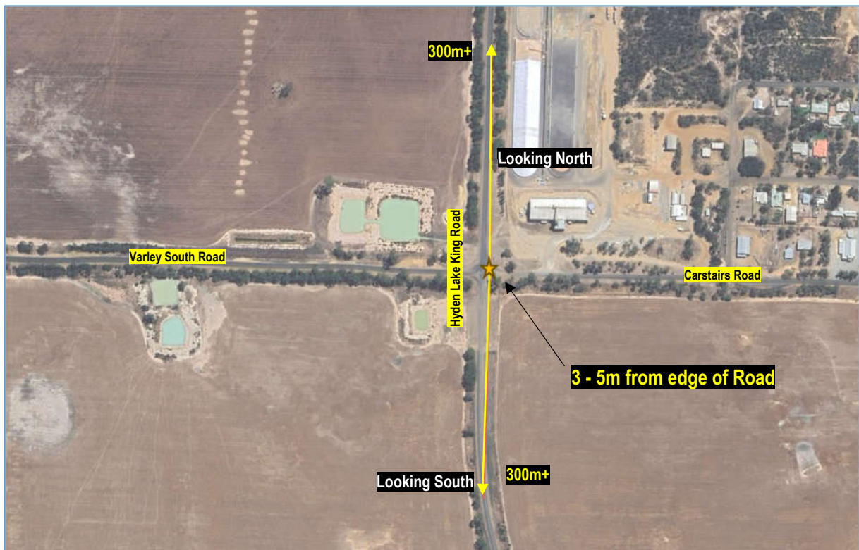
Figure 19: Sight Distance Check – Hyden Lake King Road / Varley South Road / Carstairs Road Intersection
